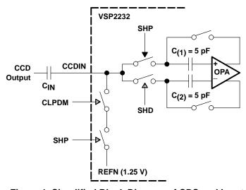
Figure 1. Simplified Block Diagram of CDS and Input Clamp
